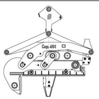
Heppenstall vertical coil tongs are designed to accommodate custom coils of all dimensions.
