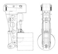
Heppenstall upender are designed to accommodate custom coils of all dimensions with or without rotating unit.
