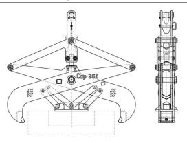
Heppenstall slab tongs are designed to accommodate custom slabs of all dimensions with or without rotating unit.
