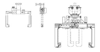
Heppenstall horizontal coil tongs are designed to accommodate custom coils of all dimensions with or without rotating unit.
